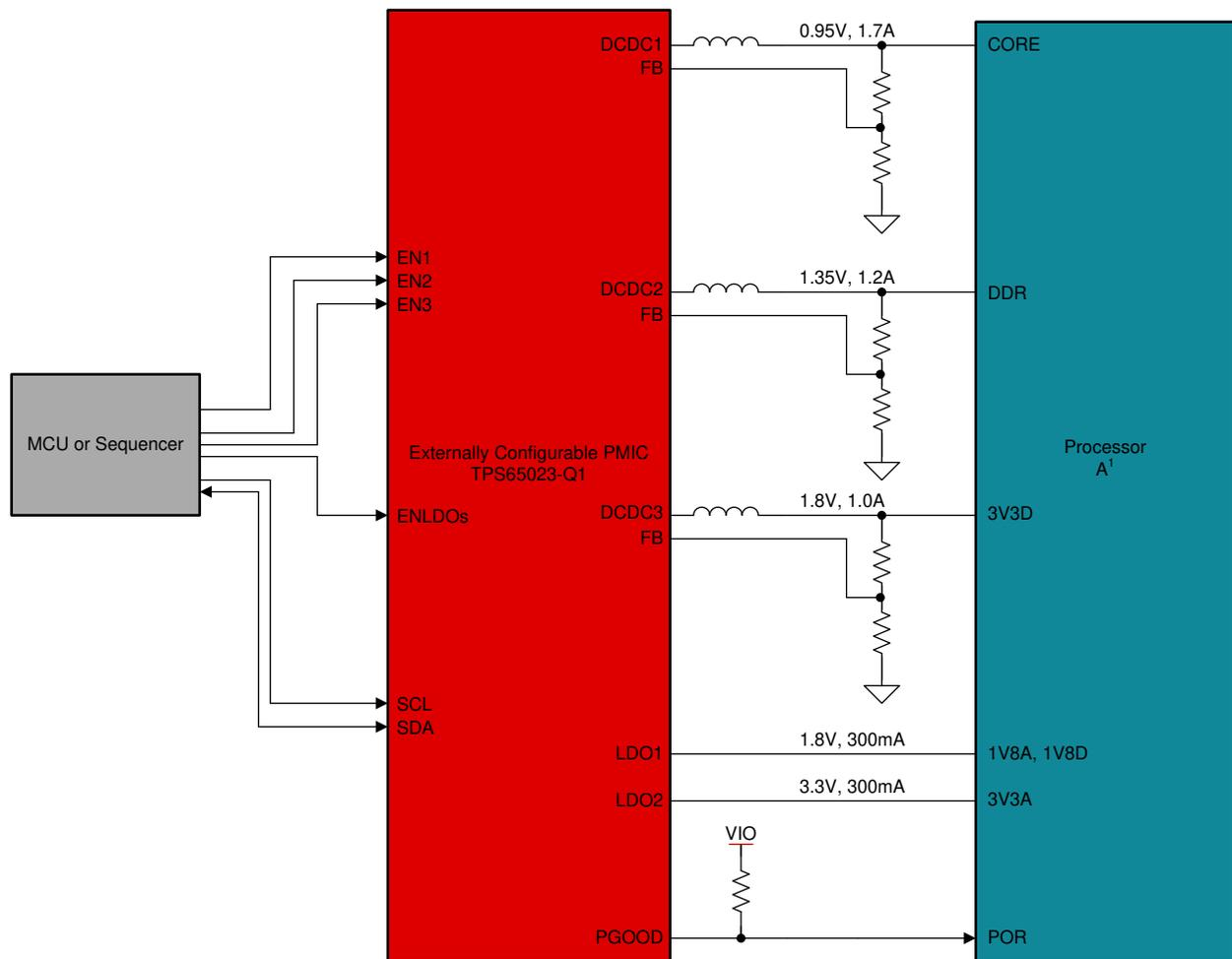
Figure 5. Hybrid (Externally Configurable PMIC) Processor Power
