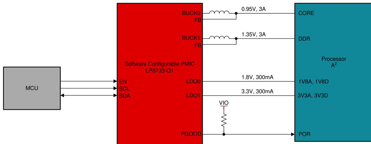
**Figure 6. Higher Current PMIC Processor Power**
