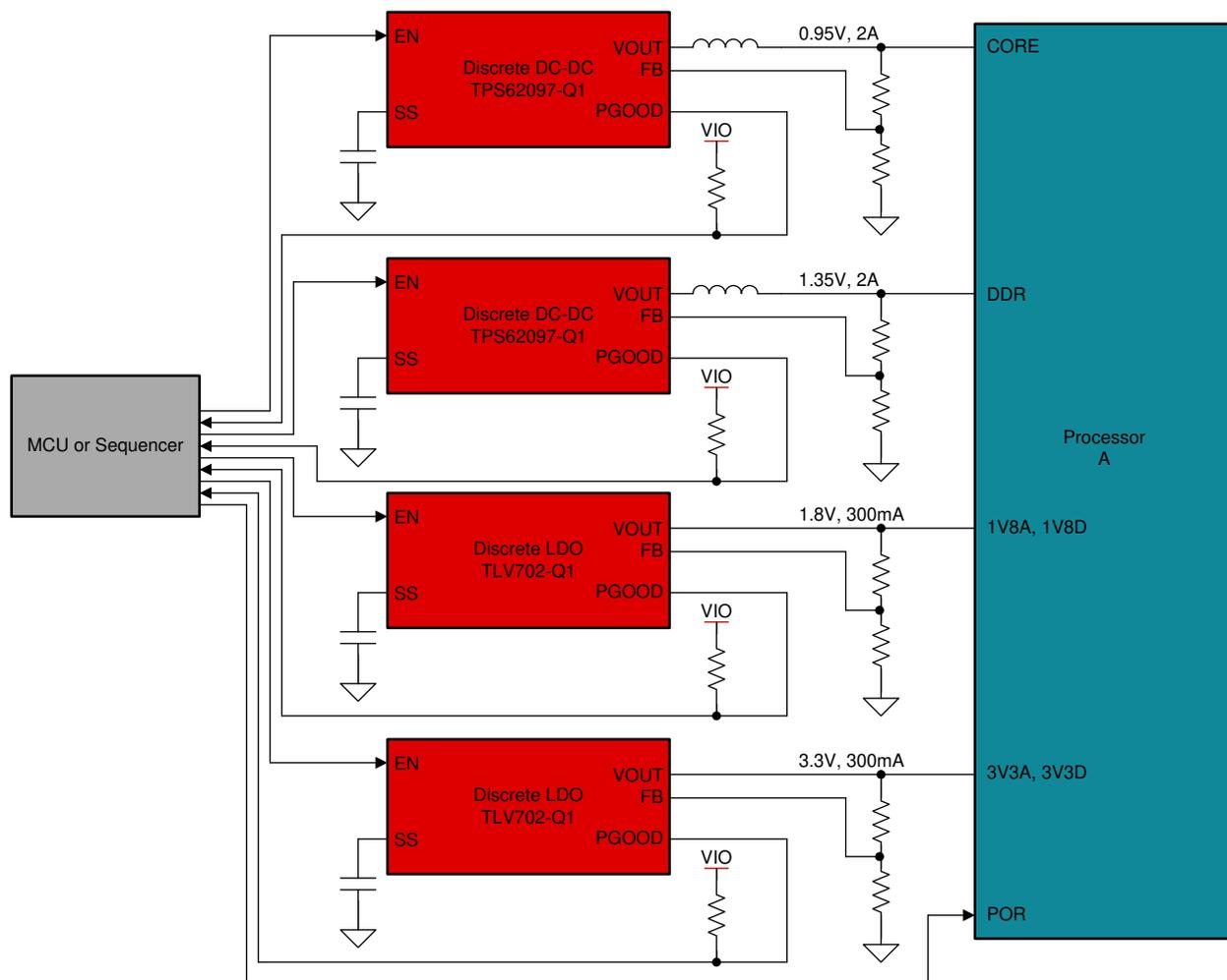
**Figure 1. Discrete Processor Power**
