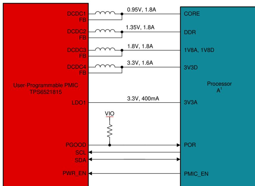
Figure 7. User-Programmable PMIC Processor Power
