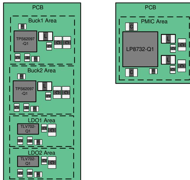
Figure 3. Example PCB Layout of Discrete versus PMIC Power Implementation
