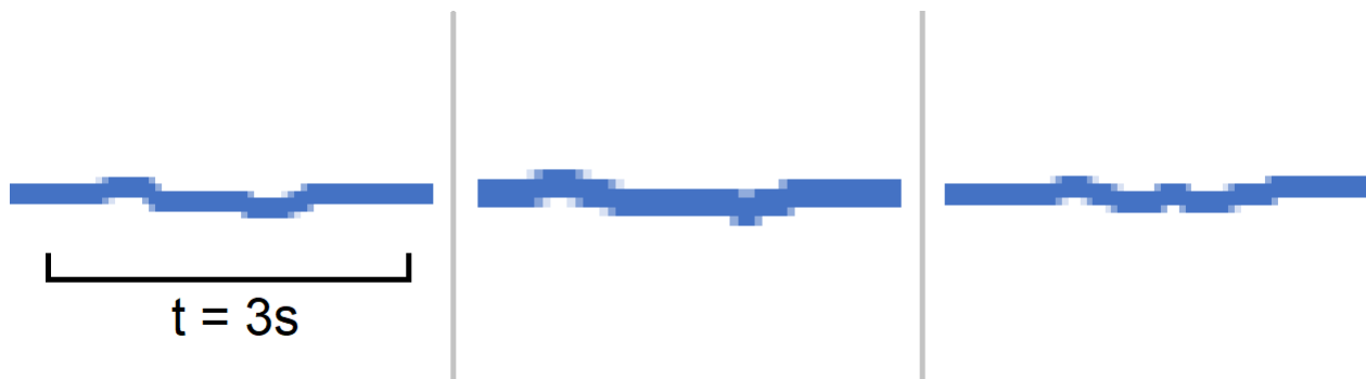
Figure 5-3. Object in Middle of FOV at Ranges of 4, 8, and 10 ft From Left to Right
