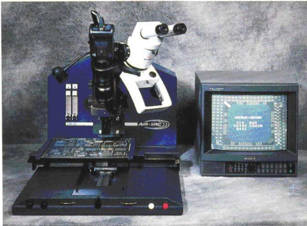
**Figure 23. DRS22C Reworking Station**
