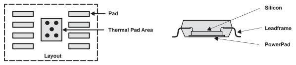
Figure 6. PowerPAD<sup>™</sup> Improves Heat Sinking
