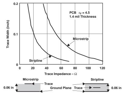
Figure 4. Trace Width on Standard PCB's
