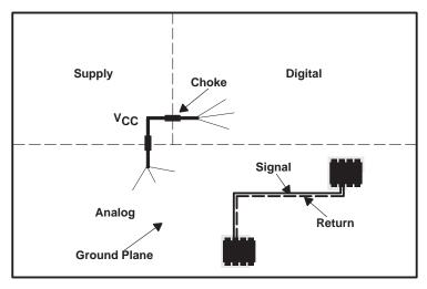
Figure 1. PCB With Proper Arrangement
