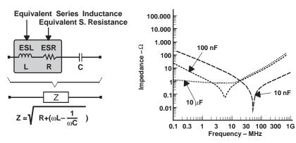
Figure 2. Impedance Behavior of a Real Capacitor
