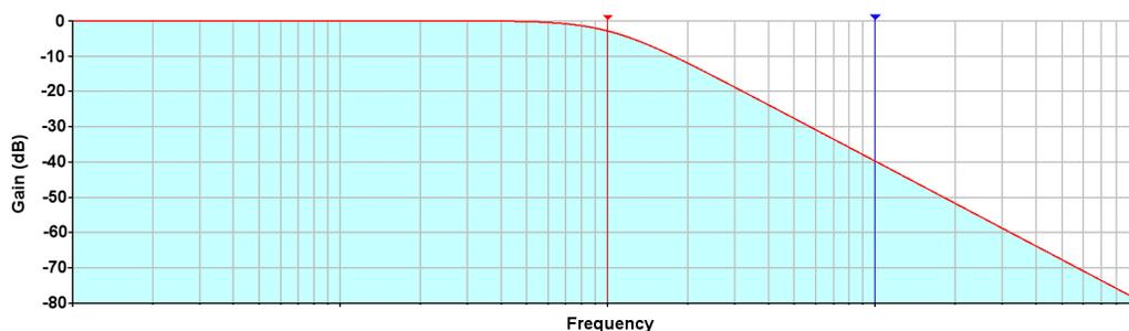
**Figure 1. Low Pass Filter Response**
