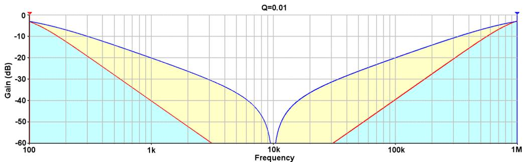
Figure 20. Q = 0.01, Notch and Band Reject Filter
