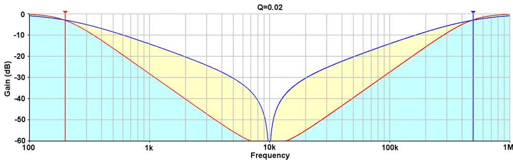
Figure 19. Q = 0.02, Notch and Band Reject Filter
