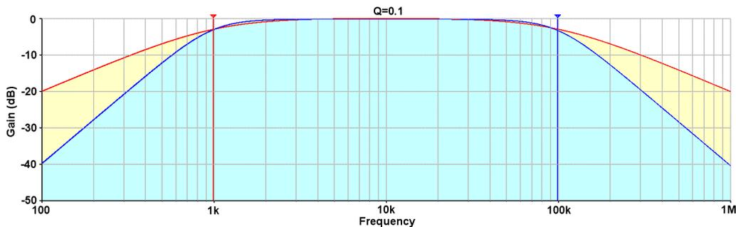
**Figure 7. Bandpass vs High Pass / Low Pass, Q = 0.1**
