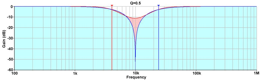
Figure 15. Q = 0.5, Notch and Band Reject Filter
