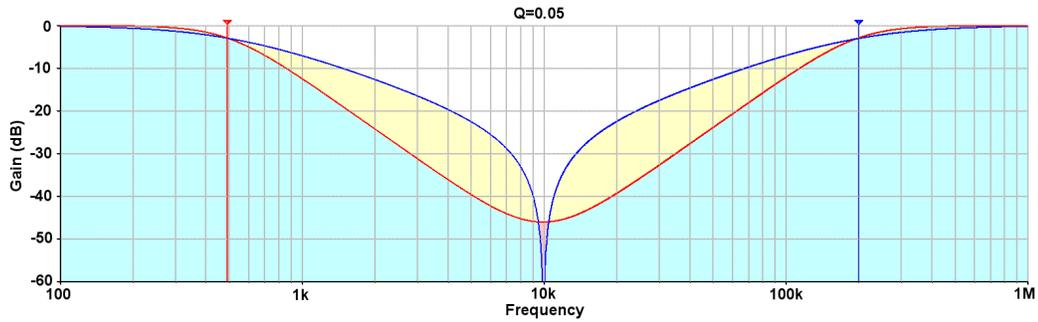
Figure 18. Q = 0.05, Notch and Band Reject Filter
