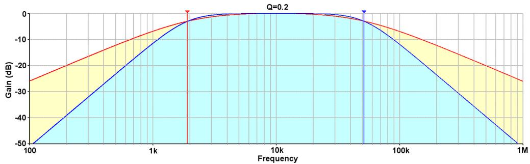
**Figure 8. Bandpass vs High Pass / Low Pass, Q = 0.2**
