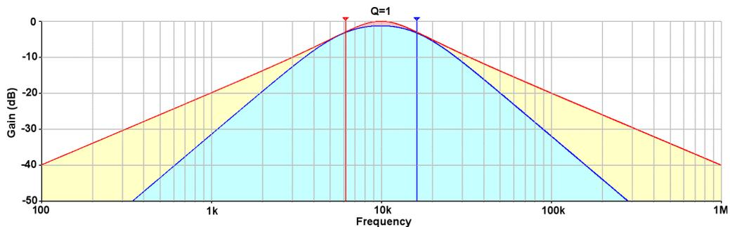
**Figure 10. Bandpass vs High Pass / Low Pass, Q = 1**
