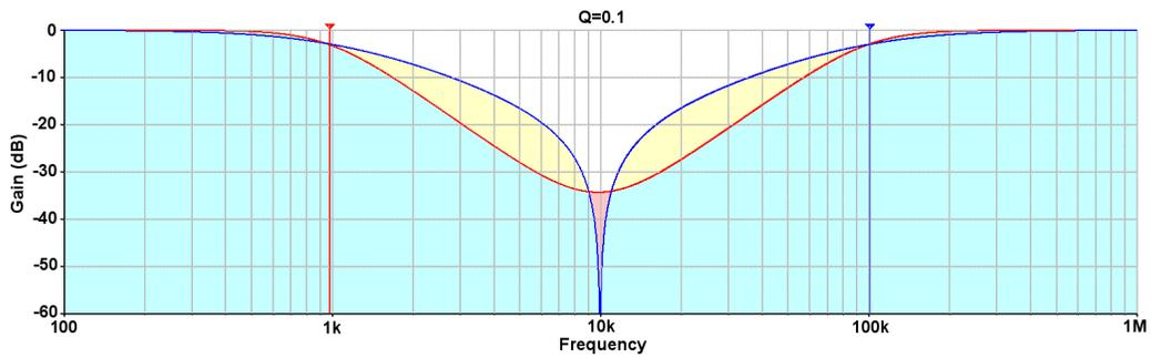
Figure 17. Q = 0.1, Notch and Band Reject Filter
