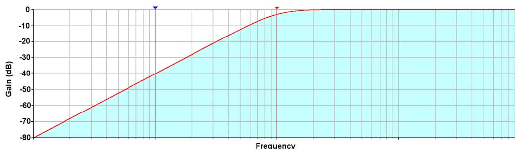
**Figure 3. High Pass Filter Response**
