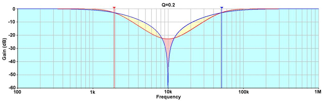
Figure 16. Q = 0.2, Notch and Band Reject Filter
