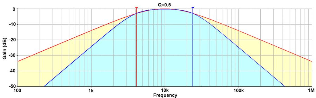
**Figure 9. Bandpass vs High Pass / Low Pass, Q = 0.5**
