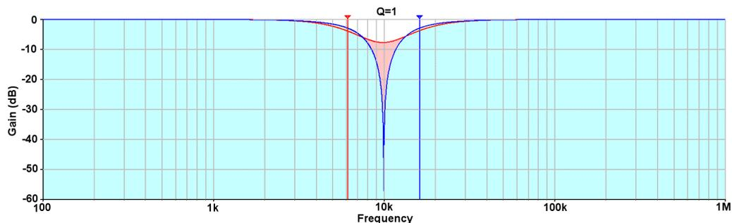
Figure 14.  $Q = 1$ , Notch and Band Reject Filter
