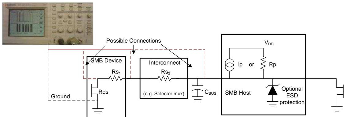
Figure 6. Different Connection Points for an Oscilloscope Trace
