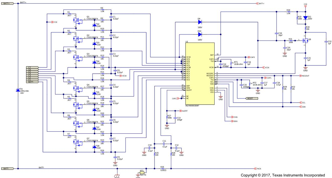
Figure 7. 7S bq76930 Configuration With External FETs
