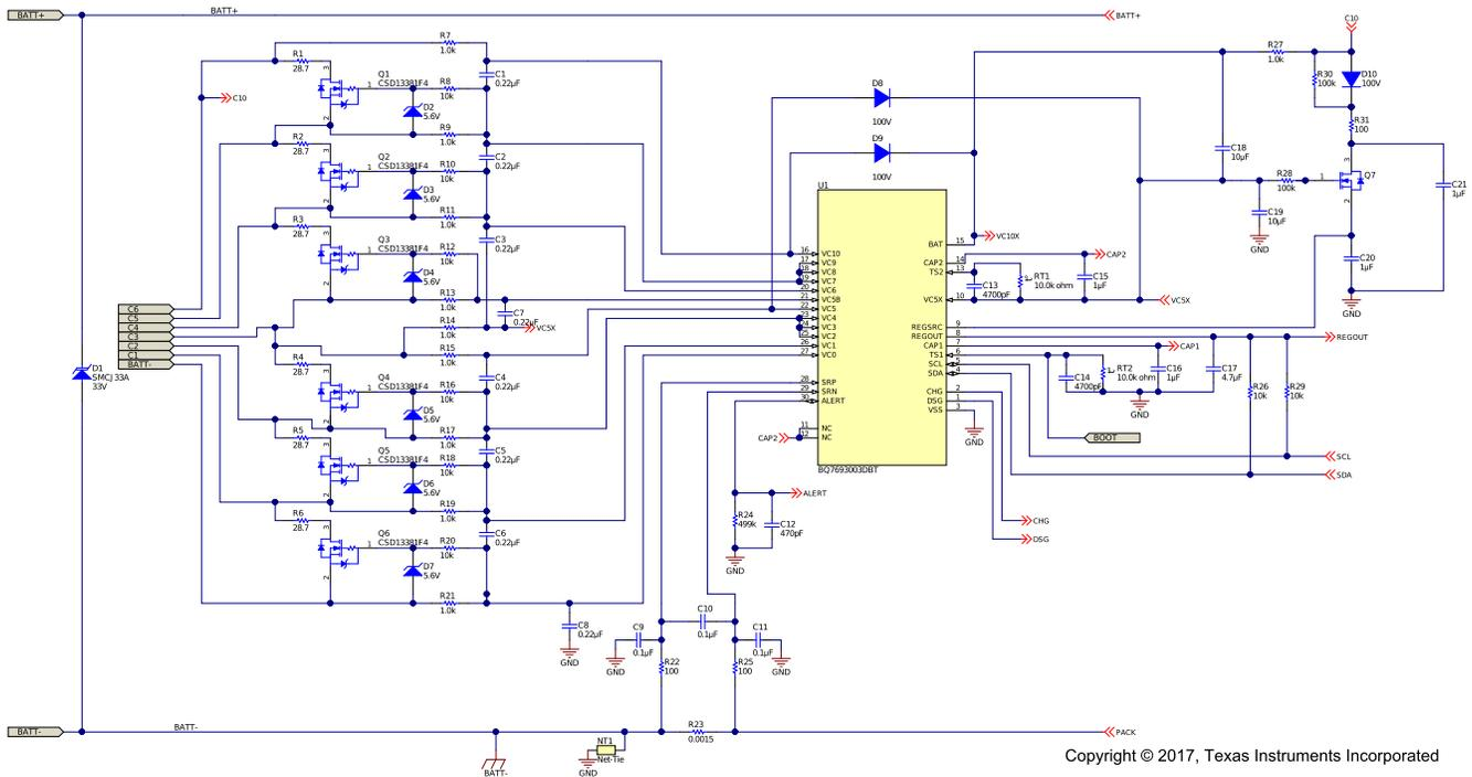
Figure 6. 6S bq76930 Configuration With External FETs
