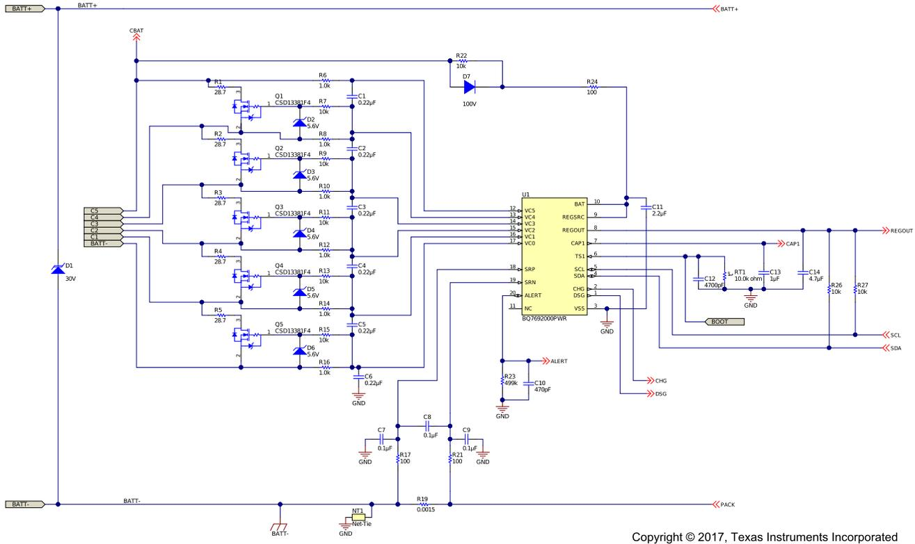
Figure 5. 5S bq76920 Configuration with External FETs
