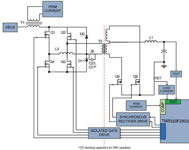
**Figure 5-1. Simplified Phase Shifted Full Bridge Converter with Secondary Side Synchronous Rectification**
