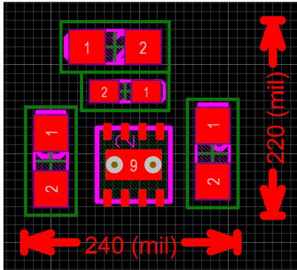
Figure 1-1. Layout Example of UCC27614 (2mm x 2mm)
