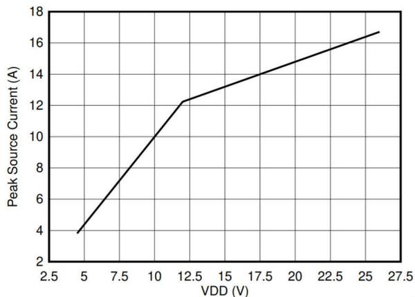
Figure 2-1. Peak Source Current vs V<sub>DD</sub>
