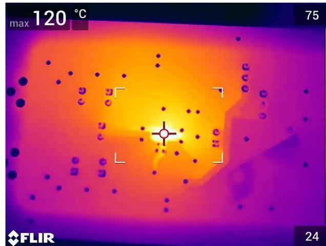
Figure 3-1. Case Temperature with  $C_{Load} = 1.8nF$ ,  $V_{DD} = 12V$ , and  $f_{sw} = 6MHz$
