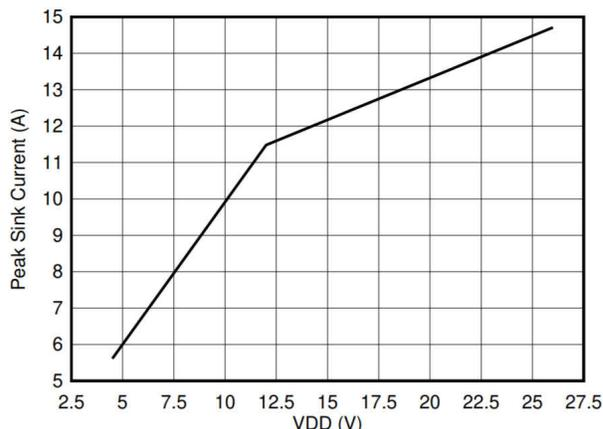
Figure 2-2. Peak Sink Current vs V<sub>DD</sub>
