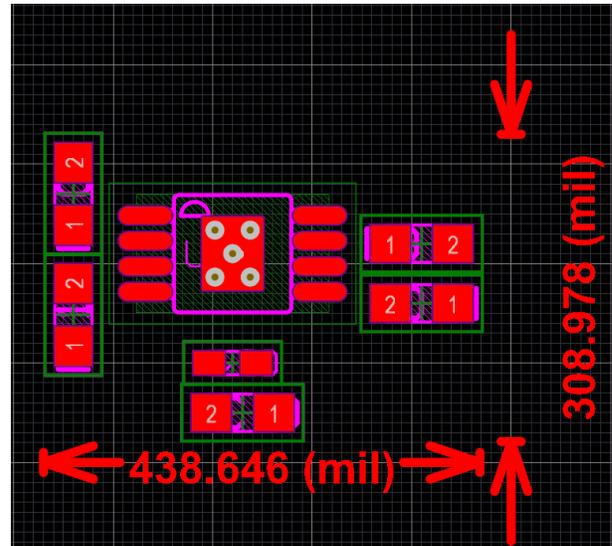
Figure 1-2. Layout Example of MSOP (5mm x 3mm) Driver
