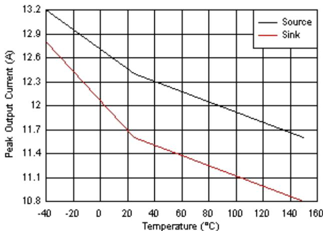
Figure 4-1. Source and Sink Current at 12 V and 100nF Load Across Temperature
