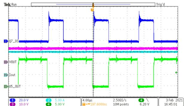
**Figure 5-3. Converter Voltage Output, Converter Current Output, Gate Drive Waveform, and MOSFET Drain to Source Voltage**
