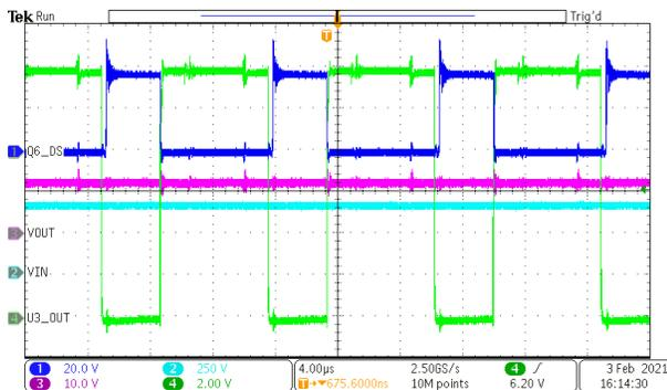
**Figure 5-2. Converter Input, Converter Output, Gate Drive Waveform, and MOSFET Drain to Source Voltage**
