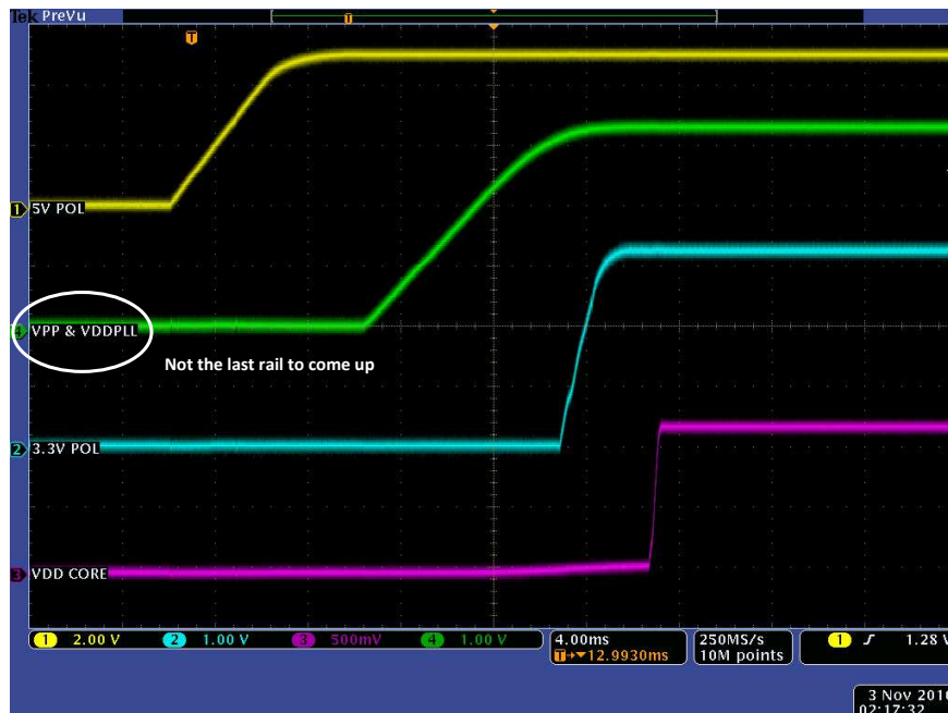
Figure 6. RTG4 Modified Development Board Fulfilling the First Power-Up Requirement
