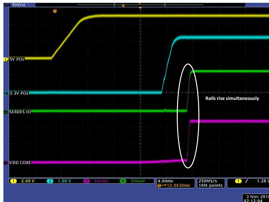
Figure 7. RTG4 Modified Development Board Fulfilling the Second Power-Up Requirement
