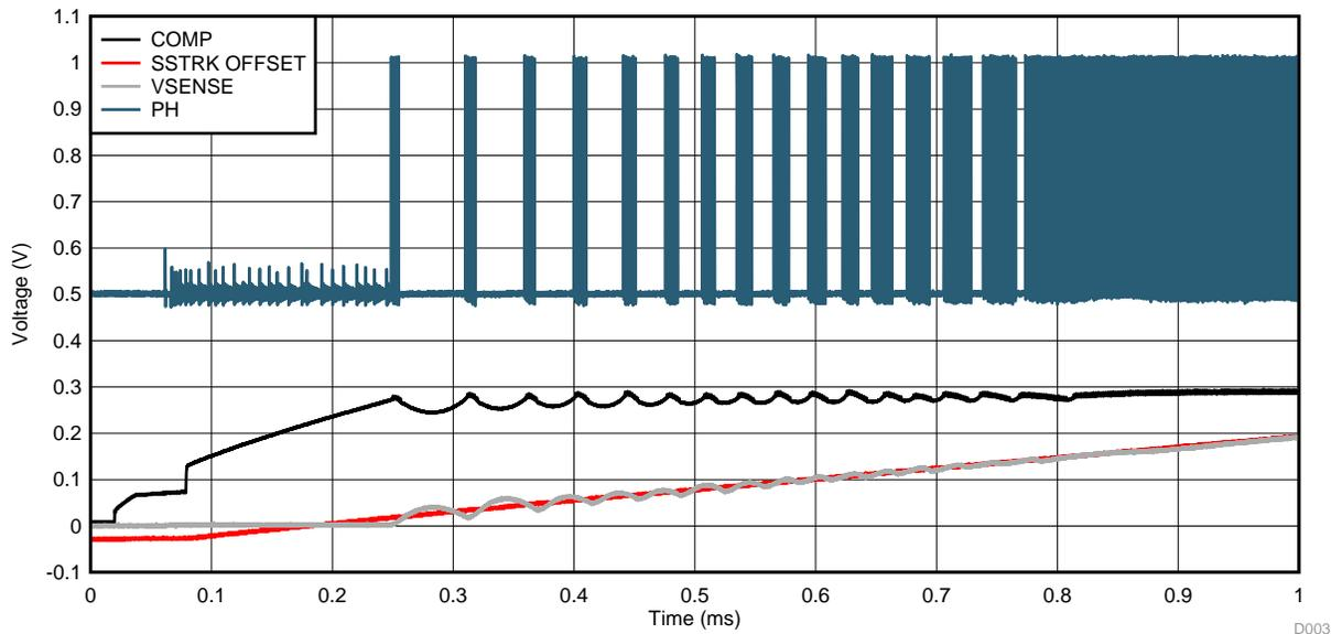
Figure 4. PH, COMP, VSENSE, and SS/TR During Startup
