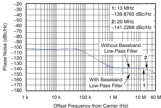
Figure 5. Measured Output Noise with and without Baseband LPF
