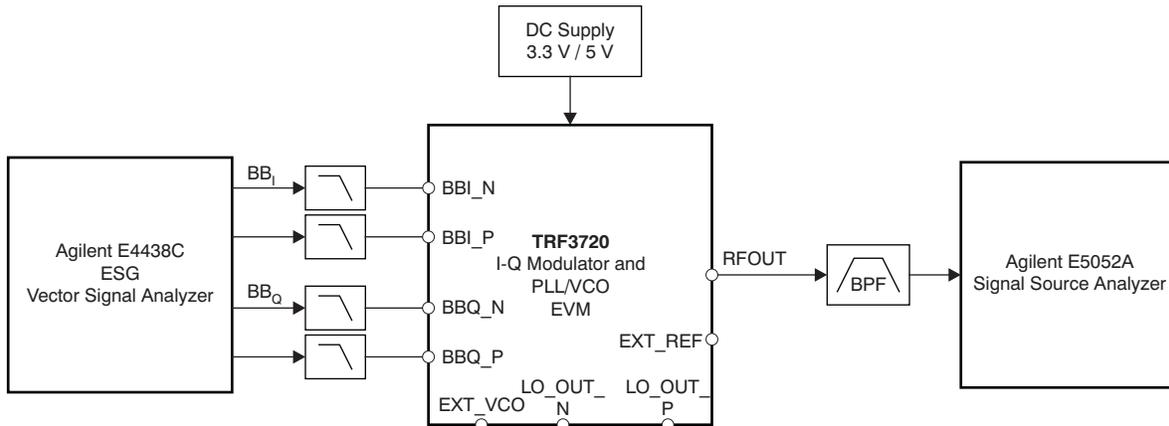
**Figure 2. Measurement Set-up to Determine Output Noise**
