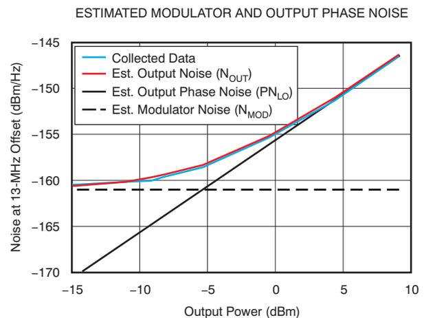
Figure 8. Estimated Modulator and Output Phase Noise for 900-MHz RF at 13-MHz Offset
