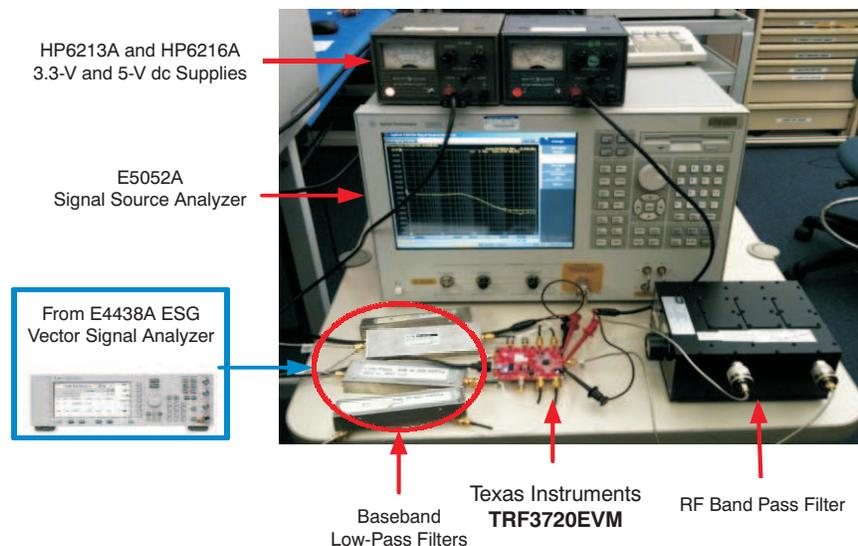
**Figure 3. Lab Measurement Set-up**
