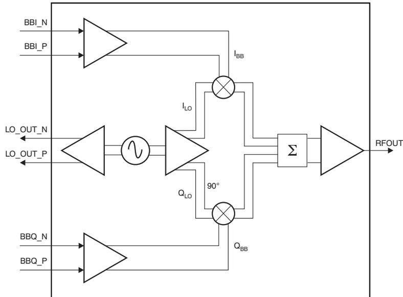
**Figure 1. TRF372017 Basic Block Diagram**
