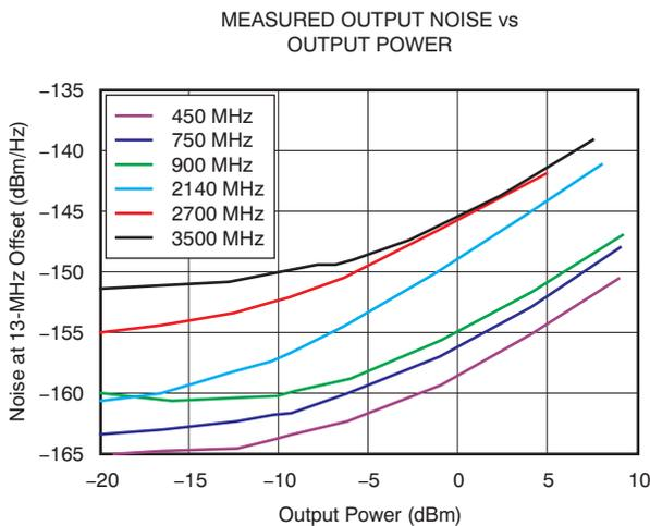
Figure 7. Measured Output Noise vs Output Power at 13-MHz Offset
