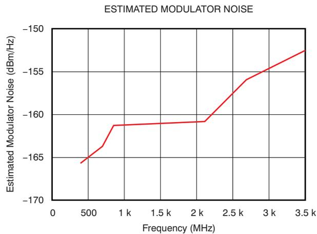
**Figure 9. Estimated Modulator Noise ( $N_{MOD}$ ) at 13-MHz Offset Across Different Carrier Frequencies**
