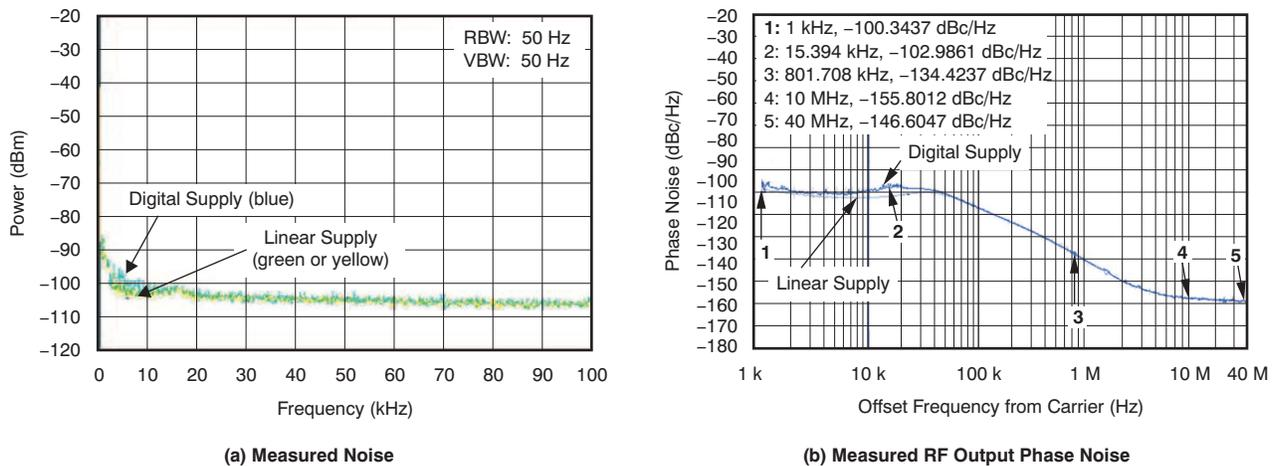
**Figure 6. Digital and Linear Supply Performance Comparison**
