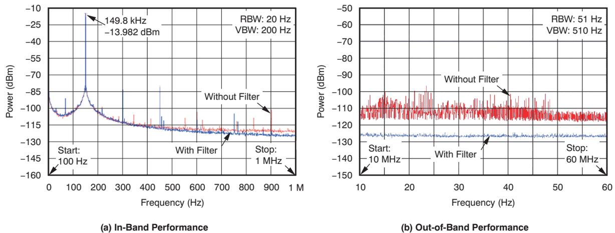
Figure 4. 150-kHz Sinusoidal Tone Response with and without Baseband LPFs
