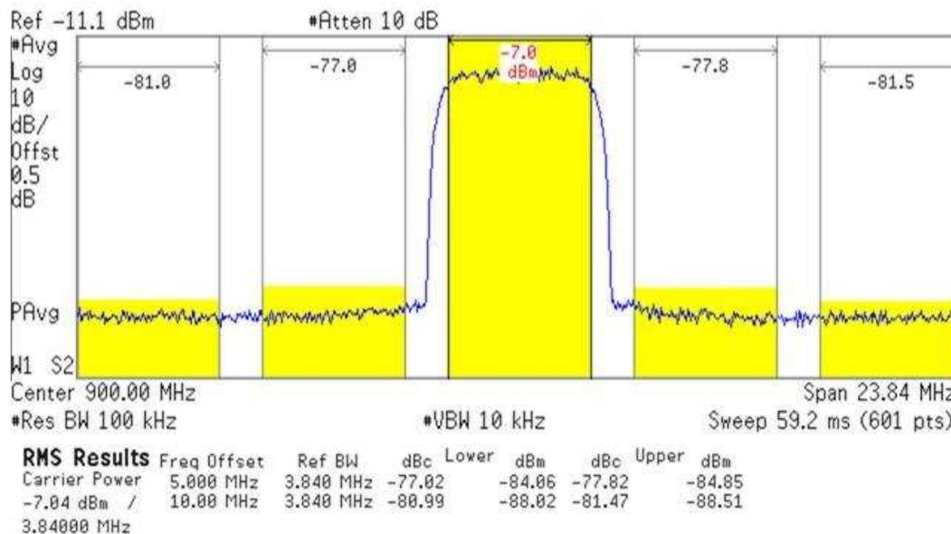
Figure 4. WCDMA Spectrum at 900-MHz LO at Zero-IF
