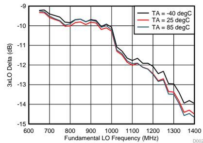
**Figure 7. 3 x LO Relative Gain versus Temperature**
