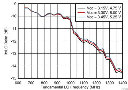
**Figure 8. 3 x LO Relative Gain versus Voltage**
