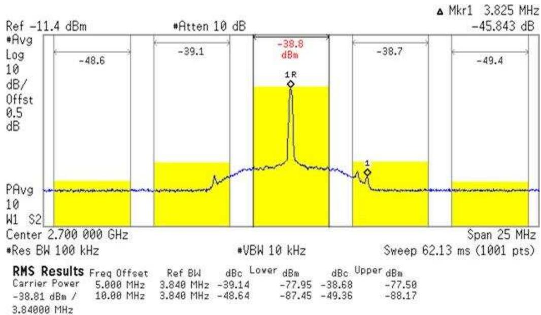
Figure 2. Baseband Distortion
