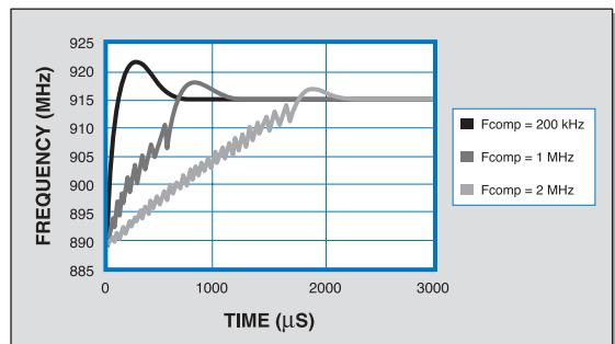
Figure 1: PLL Simulation Results
