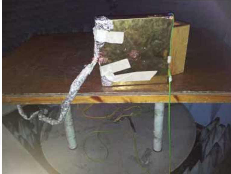
Photograph 7.1.7 Setup for radiated disturbance measurements, radiation from EUT pins
