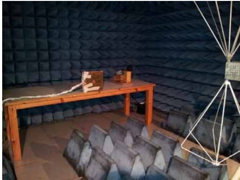
Photograph 8.1.3 Setup for radiated immunity to RF electromagnetic field test, general view, radiation from EUT pins
