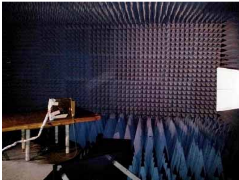
Photograph 7.1.6 Setup for radiated disturbance measurements, radiation from EUT pins
