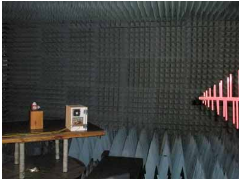
Photograph 8.1.2 Setup for radiated immunity to RF electromagnetic field test, EUT close view, EUT radiation through cable
