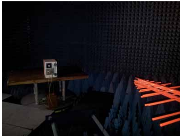
Photograph 7.1.2 Setup for preliminary radiated disturbance measurements, general view, EUT radiation through cable
