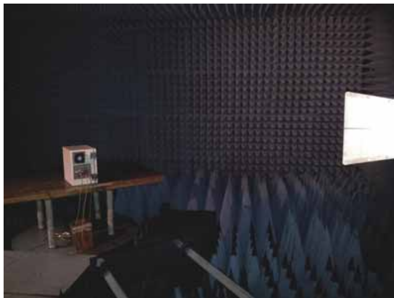
Photograph 7.1.2 Setup for preliminary radiated disturbance measurements, general view, EUT radiation through cable
