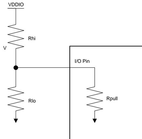
**Figure 1. Generic 4-Level Strap Diagram (Internal Pull-Down)**
