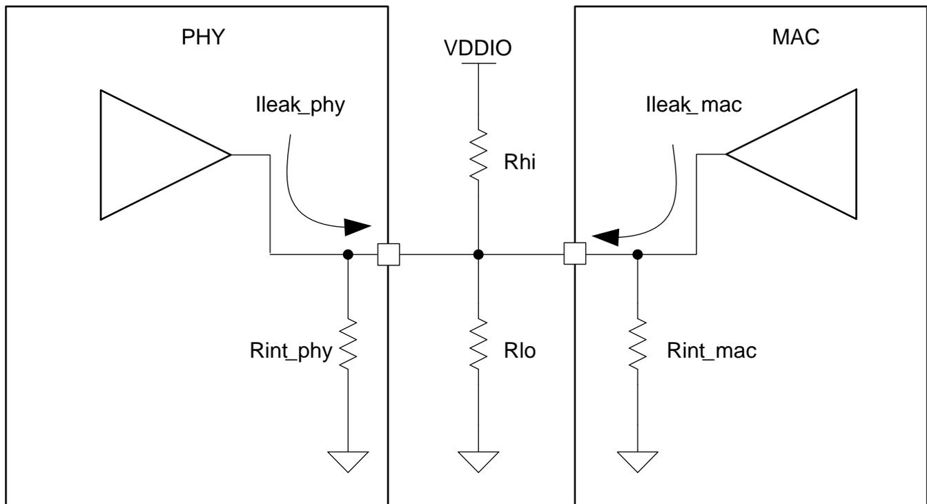
**Figure 4. 4-Level Strap Voltage Analysis Model (Internal Pull-Down)**
