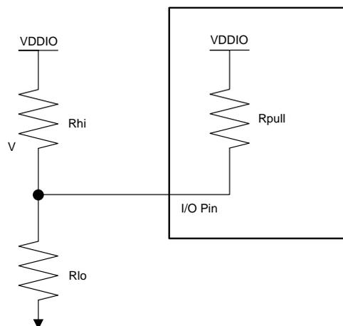
**Figure 2. Generic 4-Level Strap Diagram (Internal Pull-Up)**
