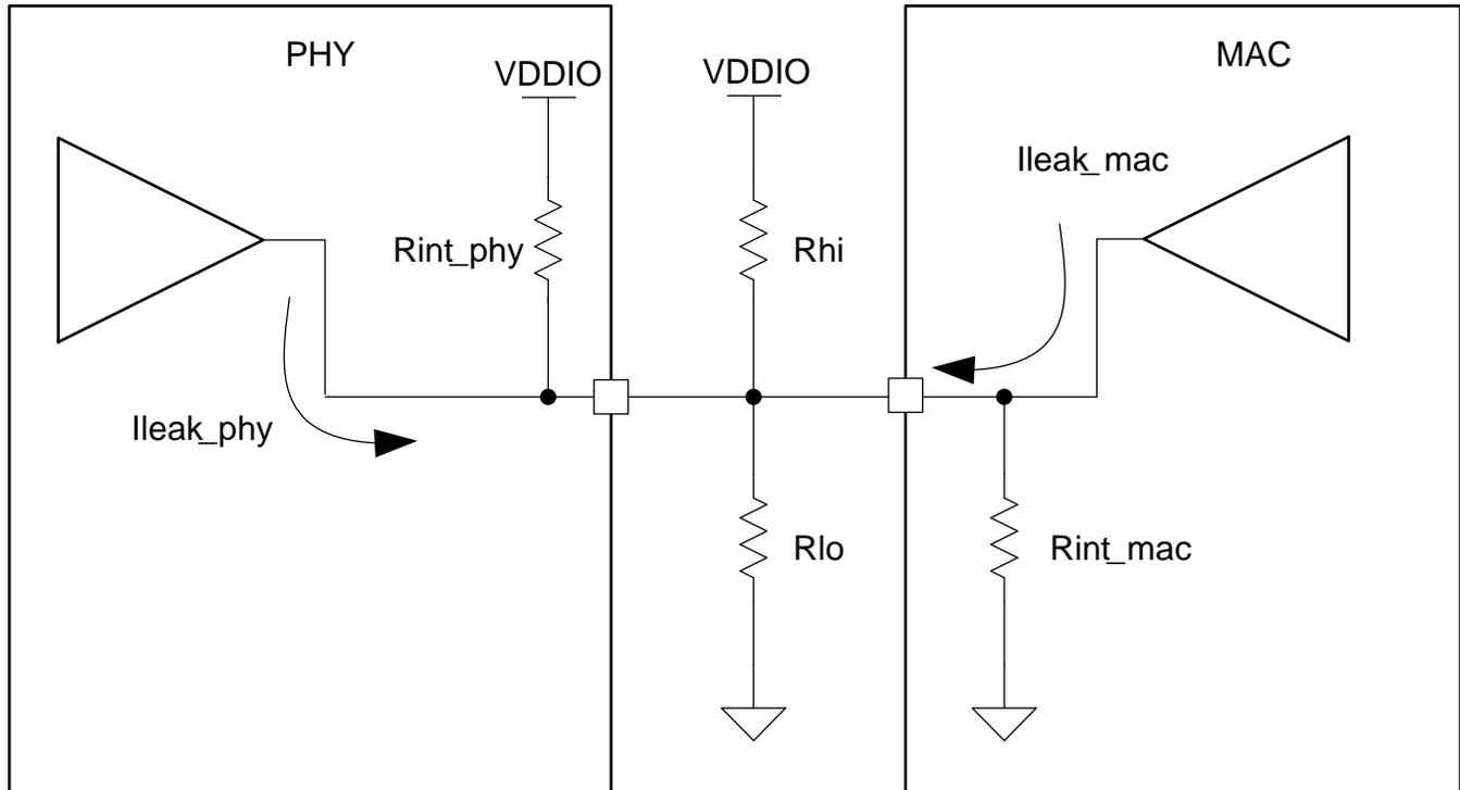
Figure 5. 4-Level Strap Voltage Analysis Model (Internal Pull-Up)
