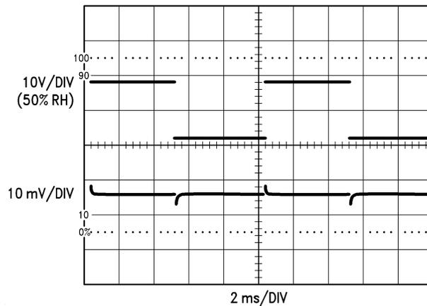
Figure 5. Humidity Sensor Waveforms
