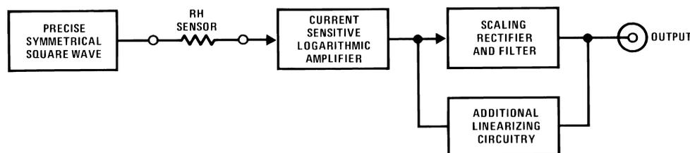
**Figure 2. Humidity Sensor Block Diagram**
