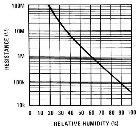
**Figure 1. Phys-Chemical Research Corp. Model PCRC-55 Humidity Sensor**
