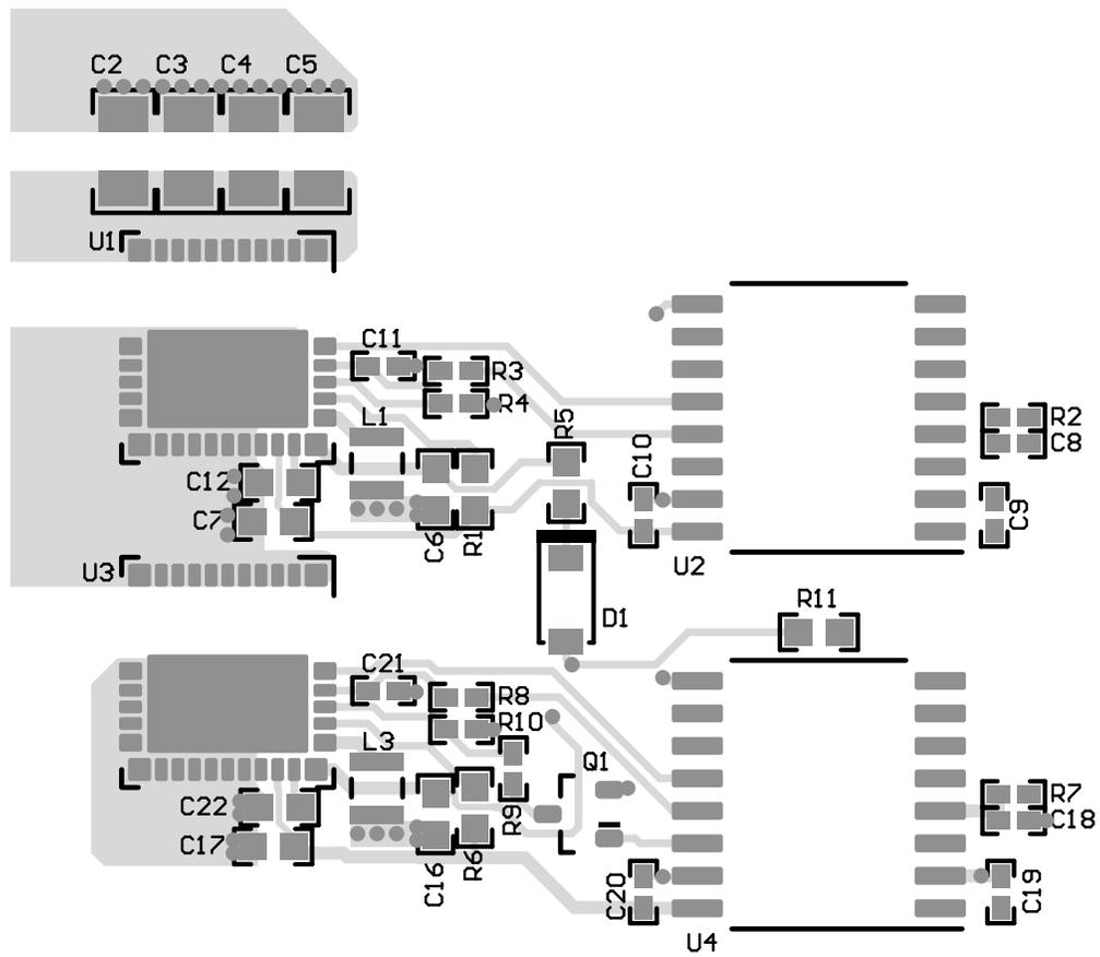
Figure 12. Top View of Example Power Stage
