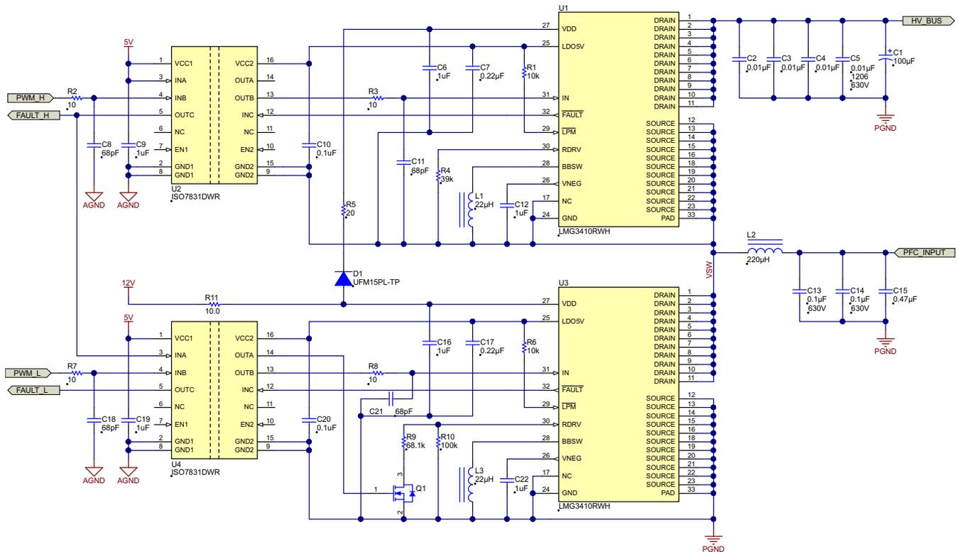
Figure 11. Schematic of Example LMG3410R070 Power Stage
