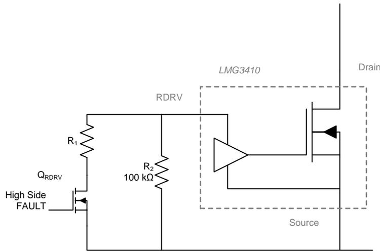
**Figure 7. LMG3410x Slew Rate Startup Adjustment Circuit**
