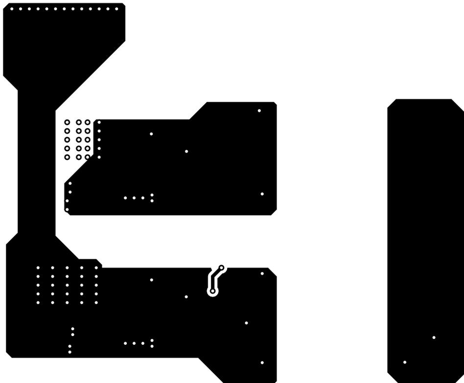
Figure 14. Mid-Layer 1 Copper of Example Power Stage
