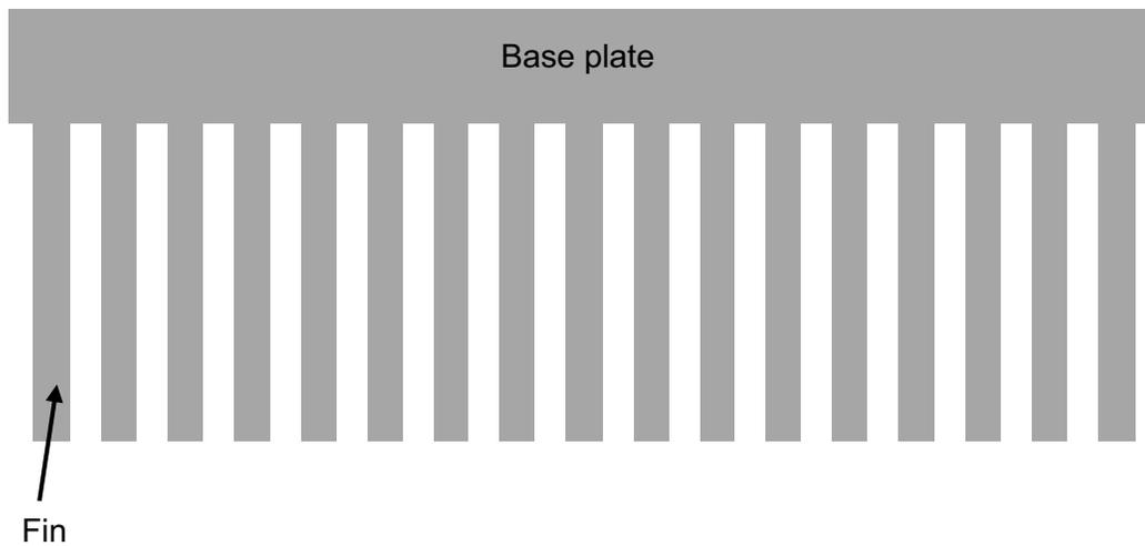
**Figure 10. Schematic of a Heatsink**
