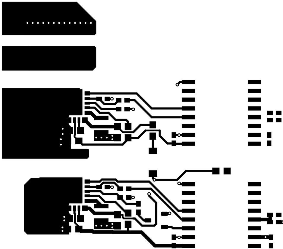
Figure 13. Top Copper of Example Power Stage
