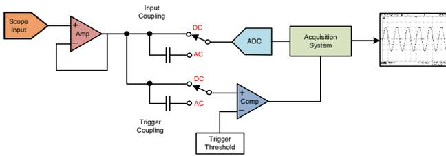
**Figure 3. Input and Trigger Coupling Block Diagram**
