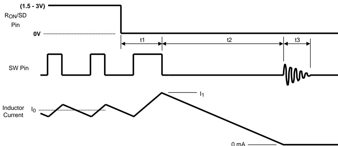
**Figure 7. Shutdown Using the  $R_{ON}/SD$  Pin**
