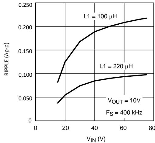
Figure 10. Inductor Ripple Current vs  $V_{IN}$  and  $L1$
