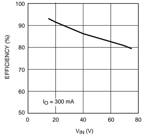
Figure 15. Efficiency at  $V_{OUT1}$  vs.  $V_{IN}$
