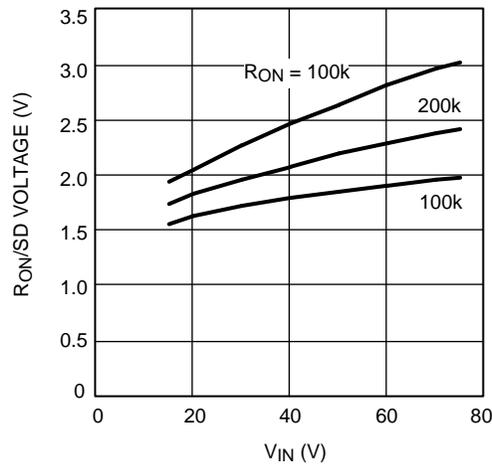
**Figure 23. Voltage at Pin 6 vs  $V_{\text{IN}}$  and  $R_{\text{ON}}$**
