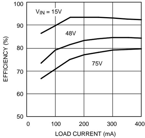
Figure 14. Efficiency vs Load Current at  $V_{OUT1}$
