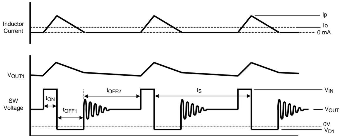
Figure 11. Discontinuous Conduction Mode
