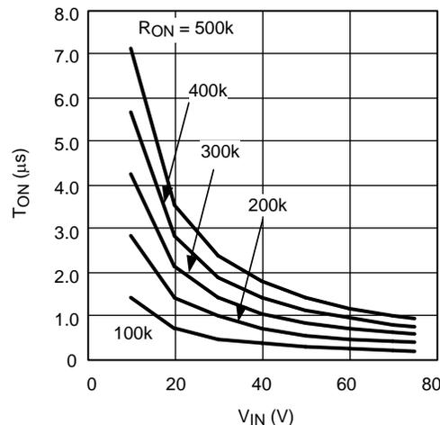
Figure 2.  $t_{ON}$  vs  $V_{IN}$  and  $R_{ON}$
