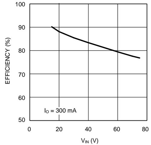
Figure 19. Efficiency vs  $V_{IN}$  at  $V_{OUT2}$
