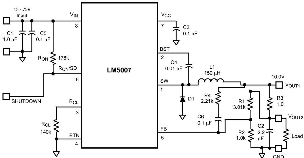
Figure 24. Low Output Ripple Configuration
