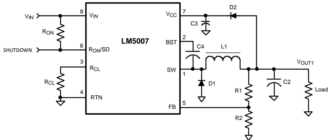
Figure 4.  $V_{CC}$  Powered by  $V_{OUT1}$
