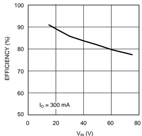
Figure 26. Efficiency vs  $V_{IN}$
