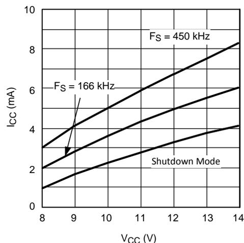
Figure 5.  $I_{CC}$  vs Externally Applied  $V_{CC}$
