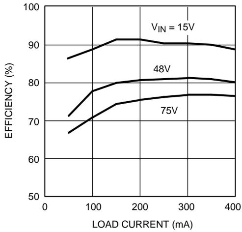
Figure 18. Efficiency vs. Load Current at  $V_{OUT2}$
