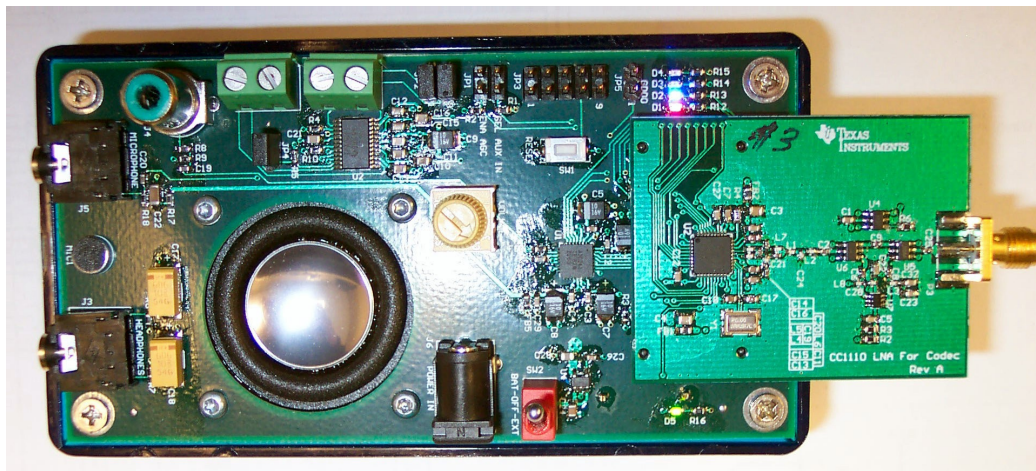
Figure 1. Two-Way Audio Transceiver with Codec (Rev B) shown with CC1110 LNA for Codec (Rev A)
