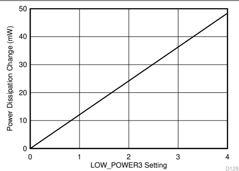
図 6-13. Power Dissipation Change vs LOW_POWER3 register setting
