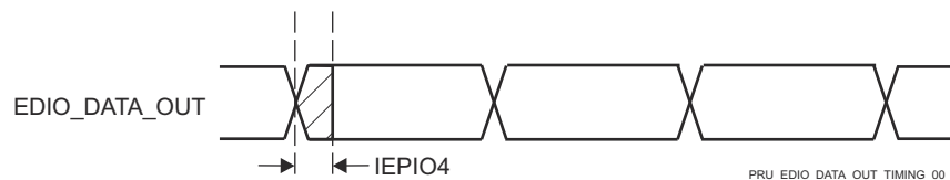
图 7-111. PRUSS IEP Digital IOs Timing Requirements
