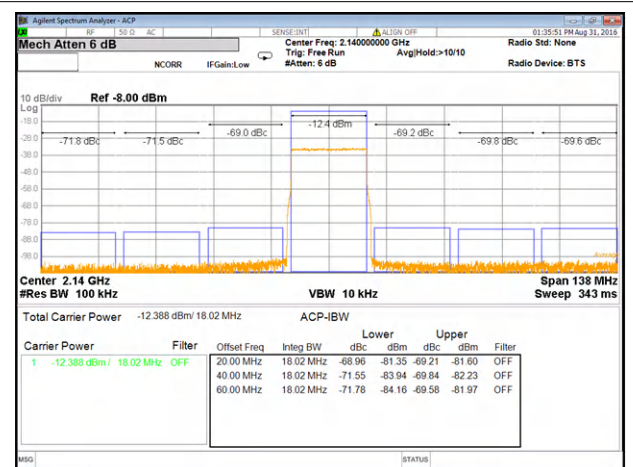
8-5. Dual band ACPR Performance in Downlink Band 1 with On-chip PLL
