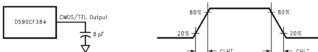
FIGURE 4. DS90CF384 (Receiver) CMOS/TTL Output Load and Transition Times
