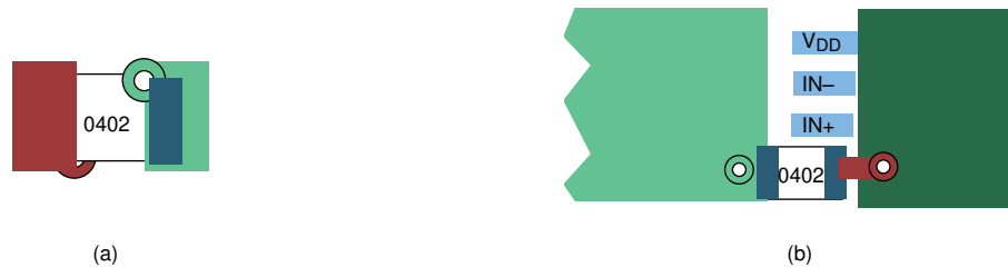
Figure 11-7. Typical Decoupling Capacitor Layouts
