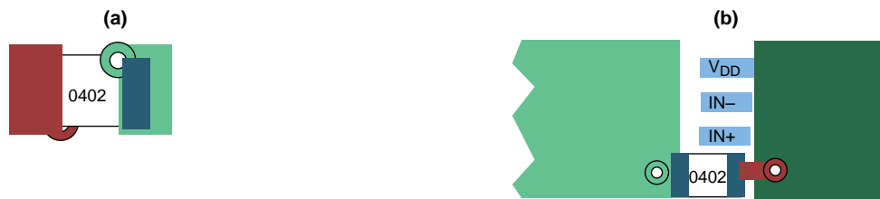
Figure 18. Typical Decoupling Capacitor Layouts
