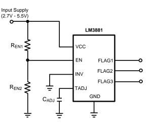
Figure 15. Enable Based On Input Supply Level
