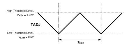
Figure 8. TADJ Pin Timing Waveform
