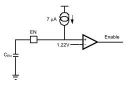
Figure 13. Precision Enable Circuit
