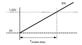
Figure 14. Enable Delay Timing
