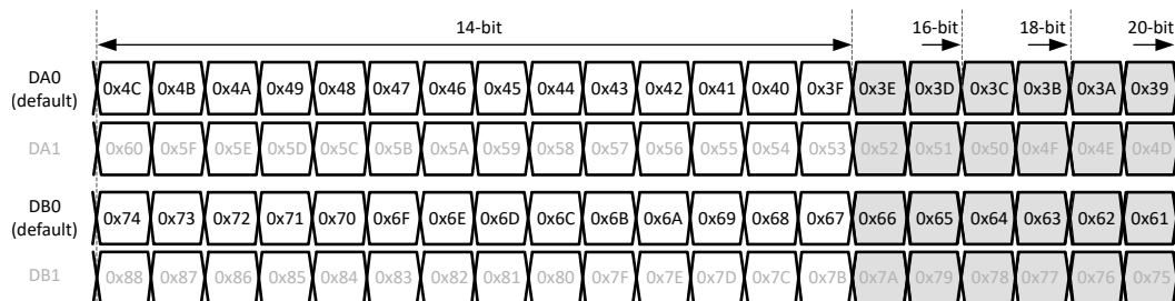
図 7-45. 1-wire output bit mapping
