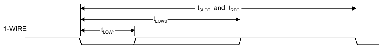
✎ 5-118. 1-Wire Write Bit Timing (Command/Address or Data)
