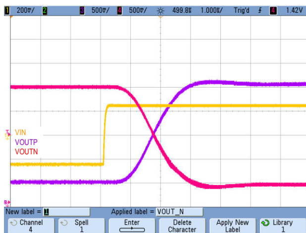
Figure 8-4. Step Response of the AMC1301
