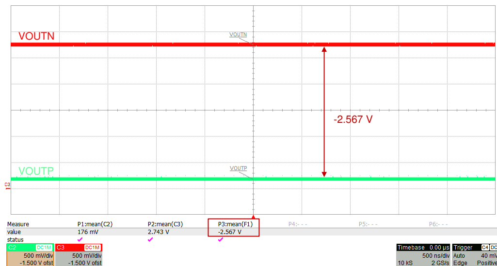
Figure 7-4. Typical Fail-Safe Output of the AMC3311-Q1
