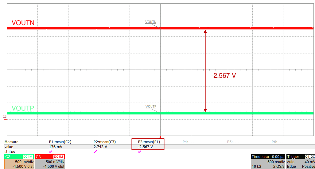
図 6-5. Typical Fail-Safe Output of the AMC3330-Q1
