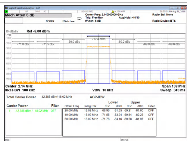
図 8-5. Dual band ACPR Performance in Downlink Band 1 with On-chip PLL
