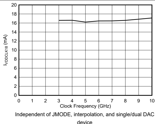
Figure 6-49. VDDCLK18 Current vs Clock Frequency
