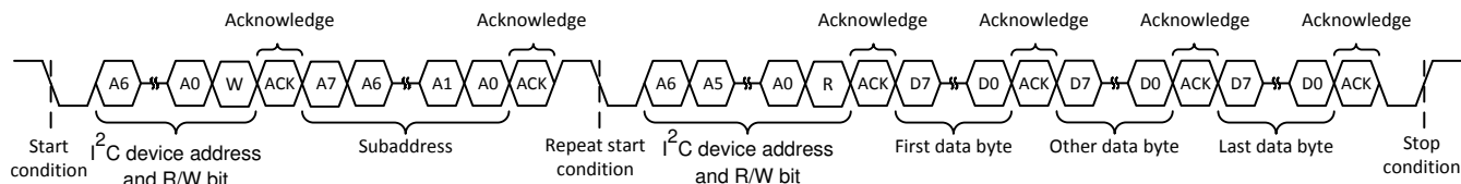
Figure 7-14. Multiple-Byte Read Transfer
