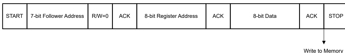
図 7-16. I 2 C Write Sequence
