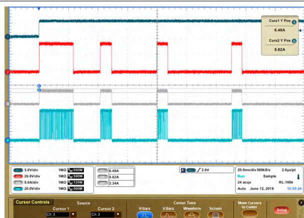
8-9. ITRIP Across TOFF and Load Current
