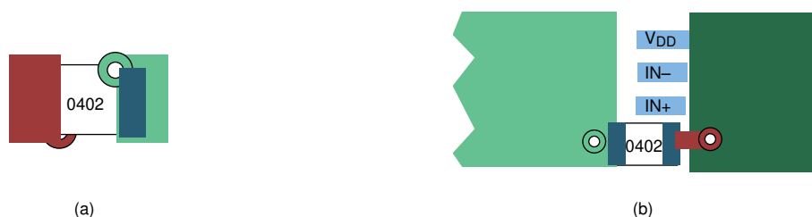
Figure 21. Typical Decoupling Capacitor Layouts
