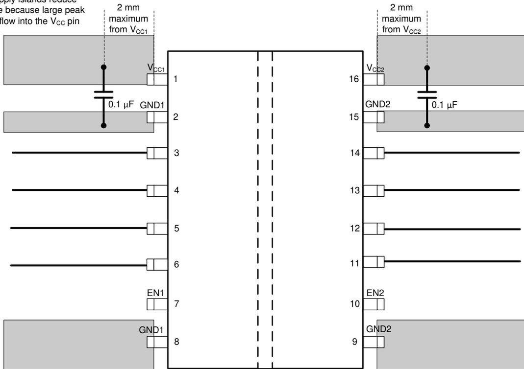
Solid ground islands help dissipate heat through PCB
