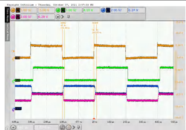
8-14. Typical TXD, RXD, CANH and CANL Waveforms at 500 kbps
