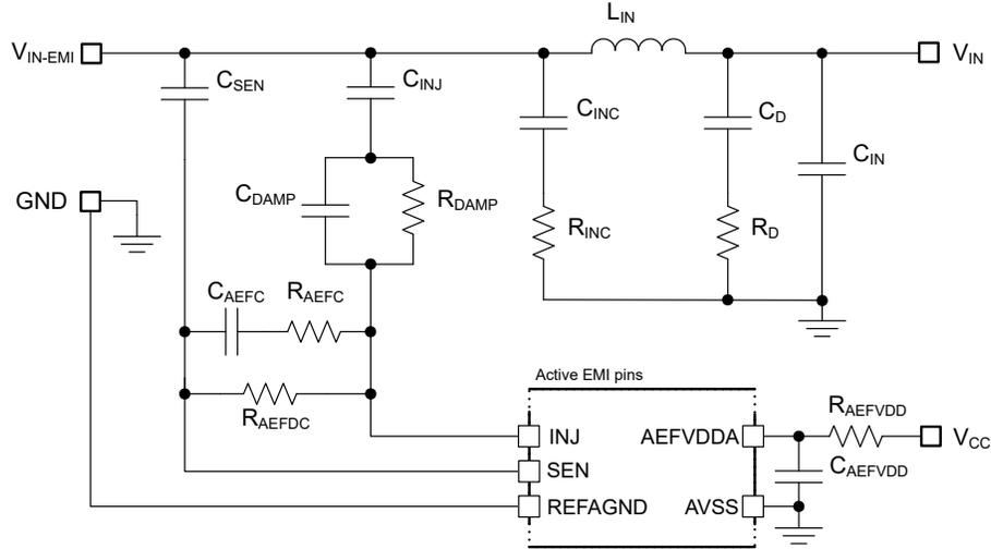
图 9-3. Active EMI Filter for a Buck Regulator
