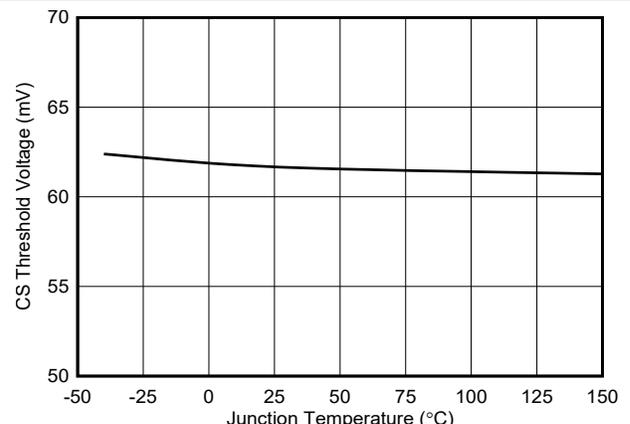
Figure 7-18. Current Sense (CS) Threshold vs Temperature
