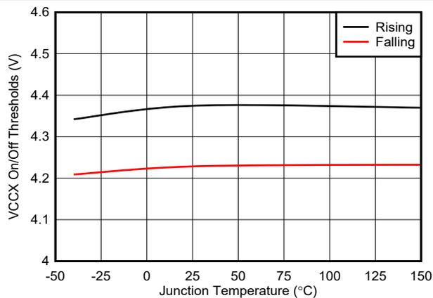
Figure 7-17. VCCX On and Off Thresholds vs Temperature
