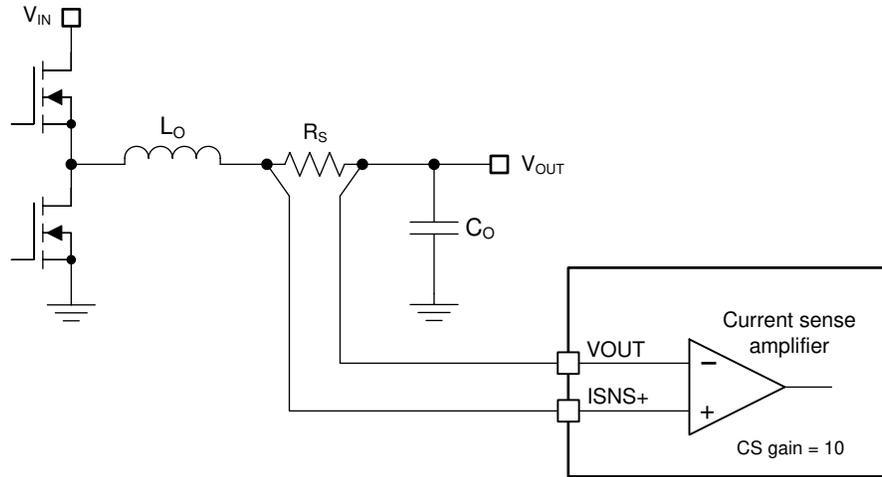
FIG 8-5. Shunt Current Sensing Implementation
