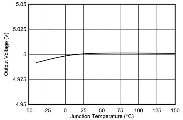
Figure 7-8. Fixed 5-V Output Voltage vs Temperature
