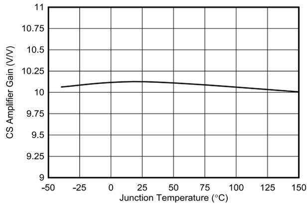
7-19. Current Sense (CS) Amplifier Gain vs Temperature
