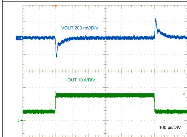
图 9-34. Load Transient, 5 A to 15 A
