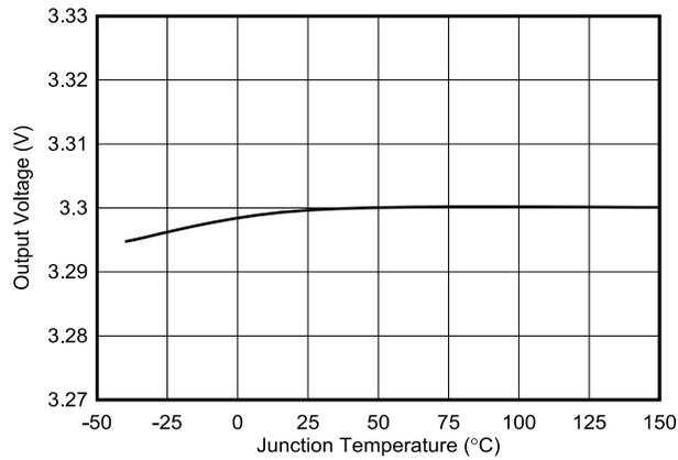
Figure 7-7. Fixed 3.3-V Output Voltage vs Temperature
