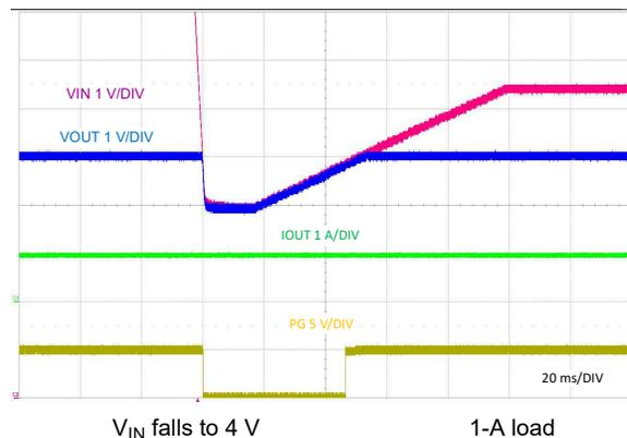
图 9-24. Cold-Crank Response to  $V_{IN} = 4\text{ V}$
