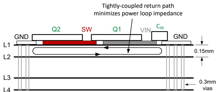
☒ 9-39. PCB Stack-up Diagram With Low L1-L2 Intra-layer Spacing <sup>1</sup>
