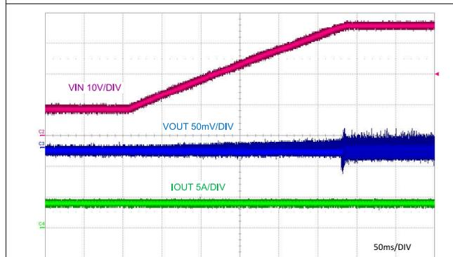
图 9-10. Line Transient Response to V<sub>IN</sub> = 36 V
