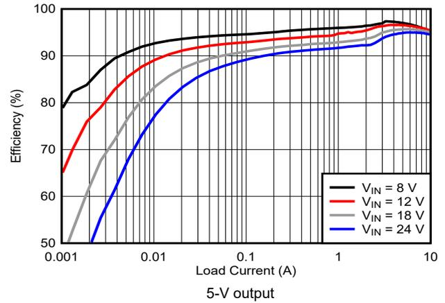
图 9-20. Efficiency vs.  $I_{OUT}$ , Log Scale
