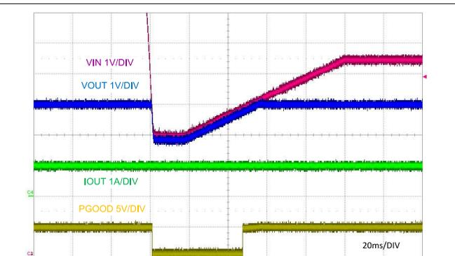
图 9-11. Cold-Crank Response to V<sub>IN</sub> = 4 V
