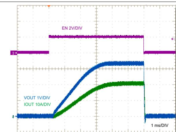
图 9-33. ENABLE ON and OFF Characteristic
