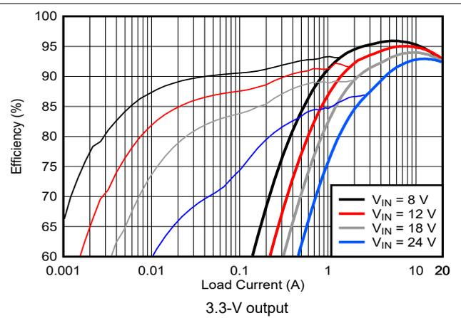
图 9-31. Efficiency vs.  $I_{OUT}$ , Log Scale
