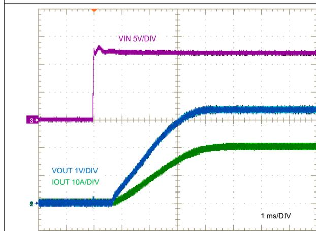
图 9-32.  $V_{IN}$  Start-Up Characteristic
