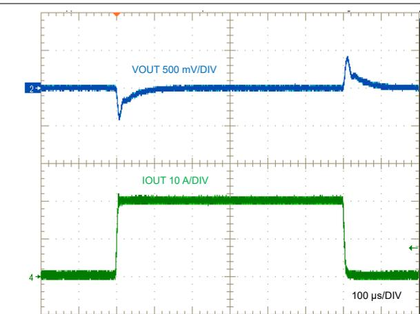
图 9-35. Load Transient, 0 A to 20 A
