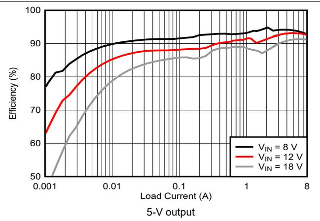
图 9-7. Efficiency vs I<sub>OUT</sub>, Log Scale
