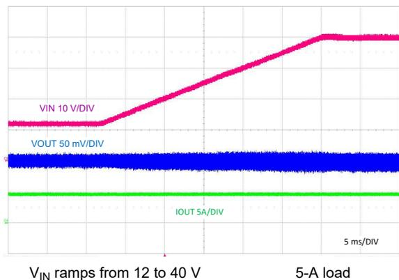
图 9-23. Line Transient Response to  $V_{IN} = 40\text{ V}$
