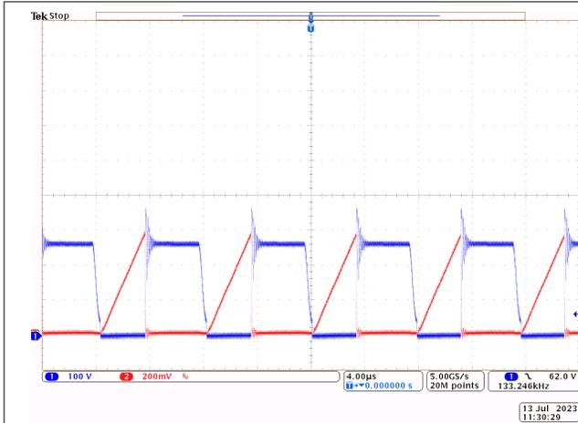
図 8-2.  $V_{IN} = 115VAC$   $V_{OUT} = 20V$   $I_{OUT} = 3.25A$
