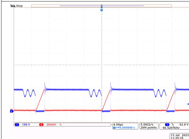
図 8-4.  $V_{IN} = 115VAC$   $V_{OUT} = 5V$   $I_{OUT} = 3A$
