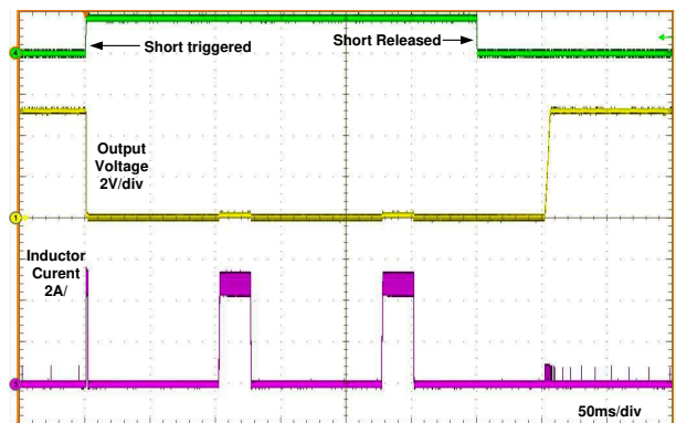
図 7-6. Short-Circuit Transient and Recovery
