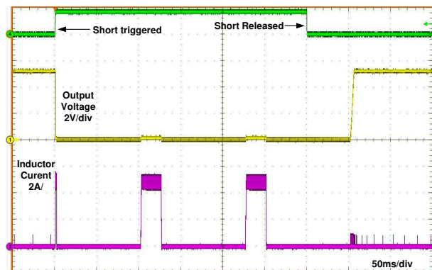
図 8-6. Short-Circuit Transient and Recovery
