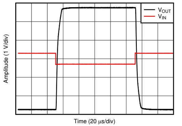
$G = -10$ ,  $V_{IN} = 600\text{mV}_{PP}$
