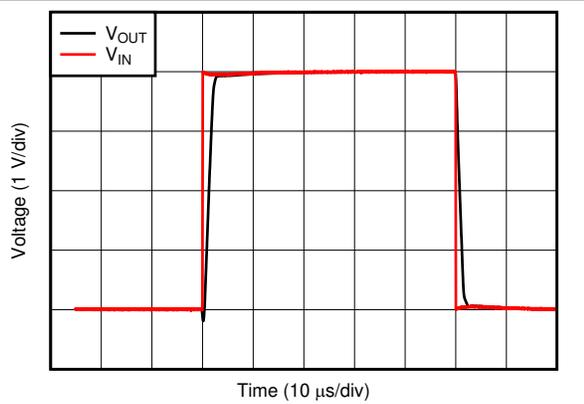
$G = 1$ ,  $V_{IN} = 4\text{V}_{PP}$ ,  $C_L = 10\text{pF}$
