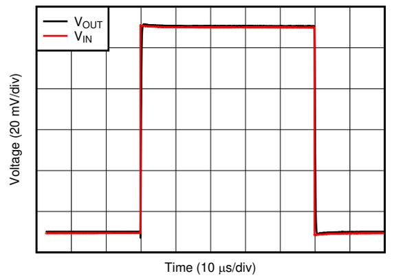
$G = 1$ ,  $V_{IN} = 100\text{mV}_{PP}$ ,  $C_L = 10\text{pF}$
