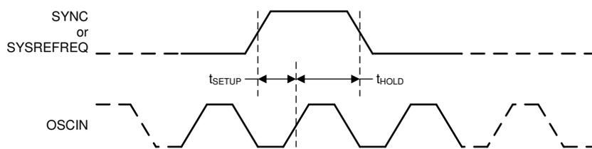
**図 6-1. Trigger Signals Timing Diagram**
