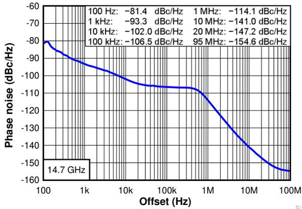
$f_{\text{OSC}} = 100 \text{ MHz}$       Jitter = 67.8 fs (100 Hz - 100 MHz)
