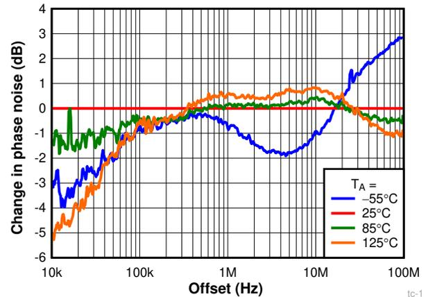
$f_{\text{VCO}} = 10 \text{ GHz}$       VCO re-calibrated at final temperature
