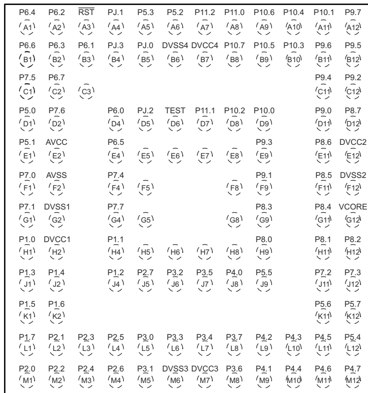
Figure 6-1. 113-Pin ZCA, GCA or ZQW Package (Top View)
