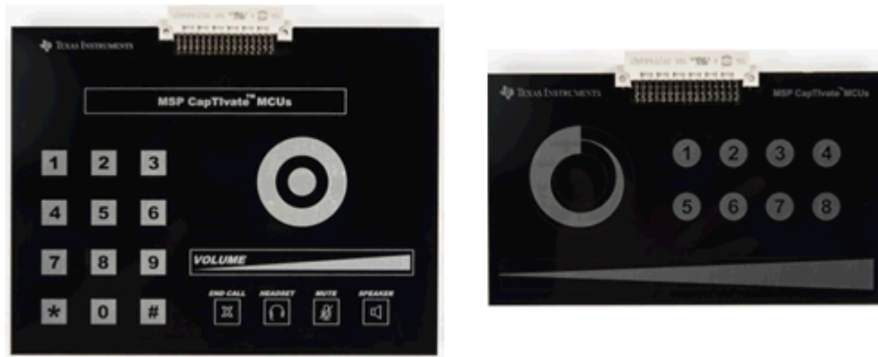
Figure 7-6. CAPTIVATE-PHONE and CAPTIVATE-BSWP Panels
