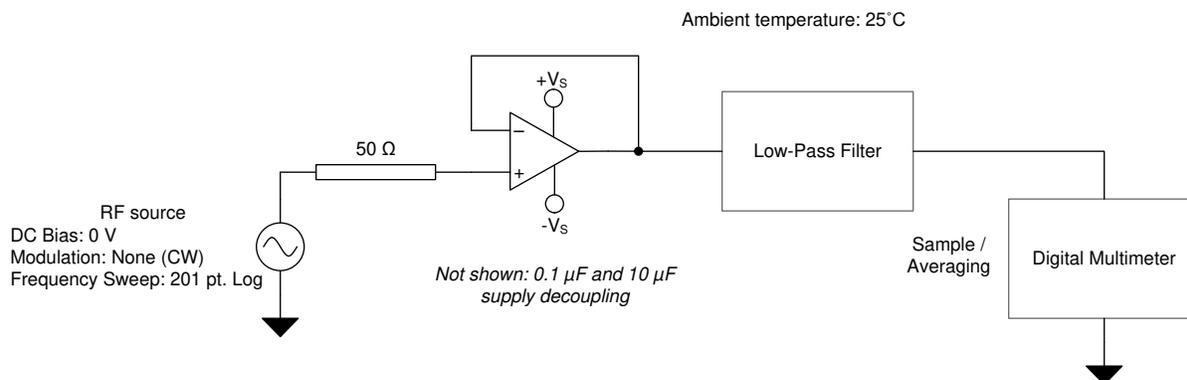
**Figure 7-7. EMIRR +IN Test Configuration**
