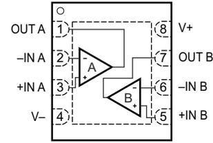
Figure 5-4. OPA2140: DRG Package, 8-Pin SON (Top View)
