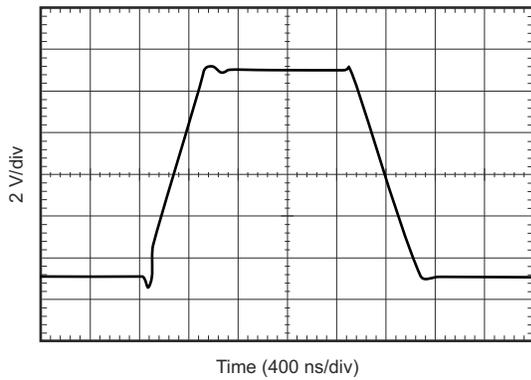
**Figure 6-29. Large-Signal Step Response**
