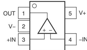
**Figure 5-2. OPA140: DBV Package, 5-Pin SOT-23 (Top View)**
