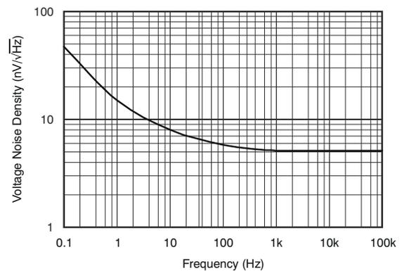
Figure 6-10. Input Voltage Noise Density vs Frequency
