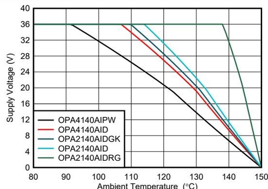
**Figure 7-4. Maximum Supply Voltage vs Temperature, DC Worst-Case**
