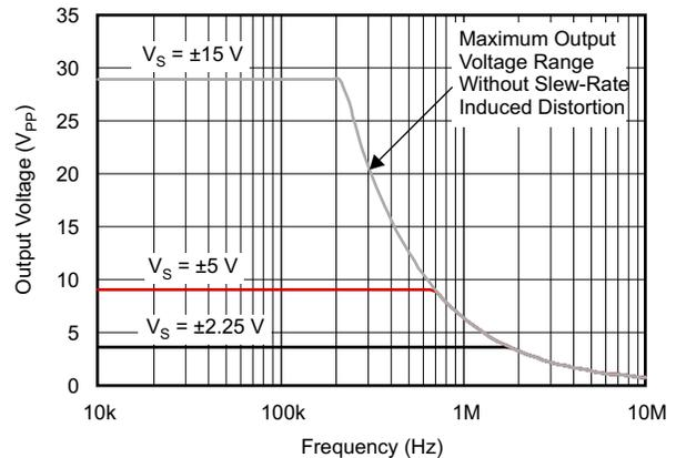
**Figure 6-22. Maximum Output Voltage vs Frequency**
