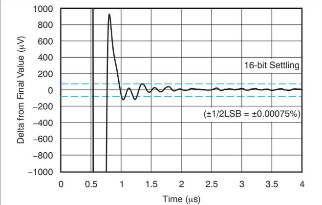
**Figure 6-26. Large-Signal Negative Settling Time (10-V Step)**
