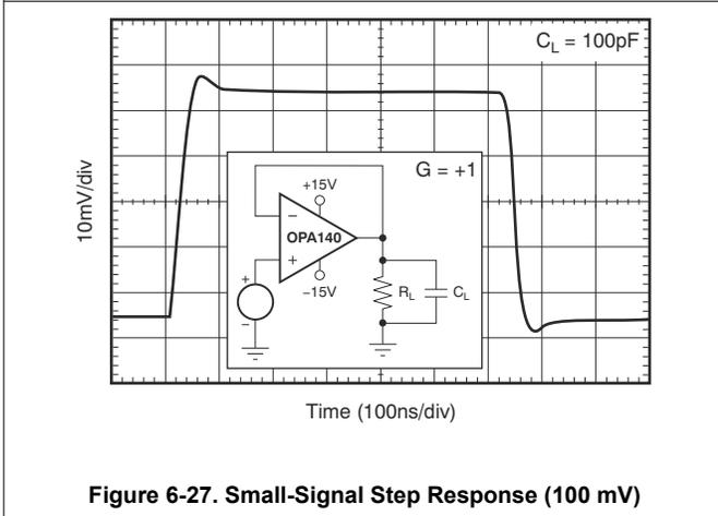
**Figure 6-27. Small-Signal Step Response (100 mV)**
