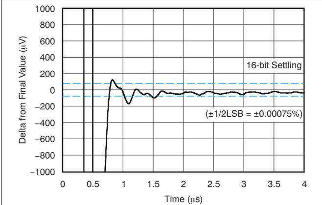
**Figure 6-25. Large-Signal Positive Settling Time (10-V Step)**
