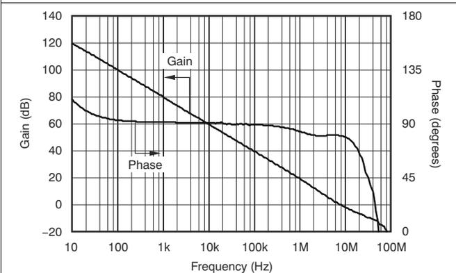
**Figure 6-15. Gain and Phase vs Frequency**
