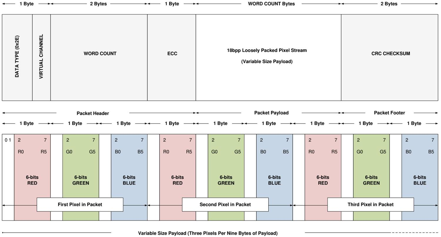
**8-7. 18 bpp (Loosely Packed) DSI Packet Structure**
