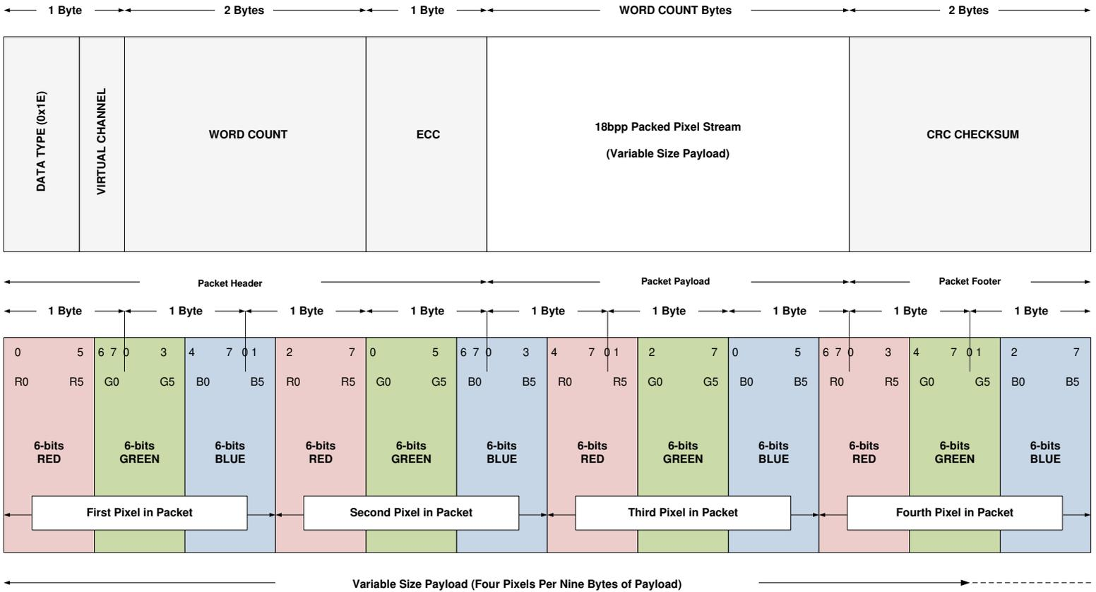
**8-8. 18 bps (Tightly Packed) DSI Packet Structure**
